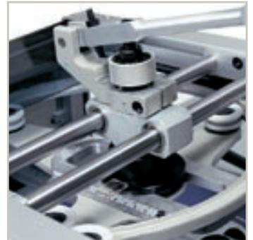
The central carriage slides on steel rods and thanks to the 2 ball bearings, its movement is very smooth which minimizes the effort of the operator.
