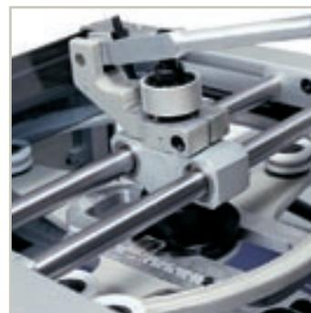
The central carriage slides on steel rods and thanks to the 2 ball bearings, its movement is very smooth which minimizes the effort of the operator.
