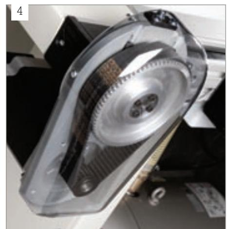
**1.** Easy and independent adjustable blade depths on each head. **2.** Digital electronics coupled with linear bearings ensure precise cutting paths and perfect results. **3.** Heavy duty and robust cutting head and mount. **4.** Powerful, quiet micro stepper motors effortlessly drive the cutting head. Components of the motor, the motor pulley and belt can be seen through the clear cover.
